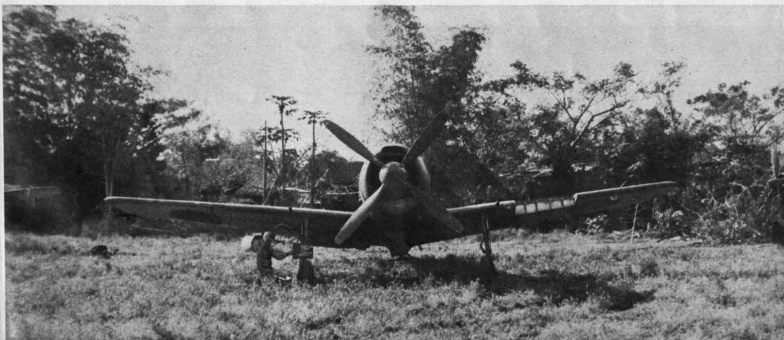
Powerful engine requires four-bladed propeller and gives Frank more prominent nose than most Jap fighters. Oval cowling is broken by air-
